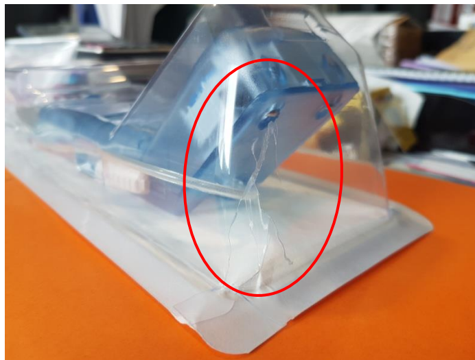
Picture 2 : Example of crack observed near the DOLPHIN inflation device pressure gauge
