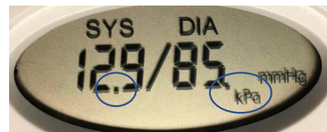
Incorrect display shows additional decimal places and kPa symbol.
