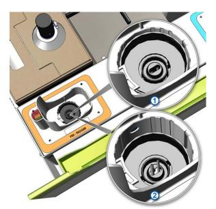
Drawing of Alinity's System pre-trigger solution bottle holder showing detail of exposed piercing probes.
