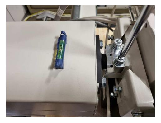
Release locking plier and reposition the end run bumpers on column and rails
