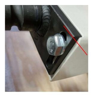
Remove the three fixing screws before the lateral ones, then the middle one
