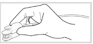
Figure 2-5: Grasping the Fiber-Optic sensor connector
