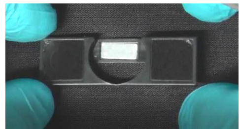
Manipulate the magnet protection without touching adhesive areas
