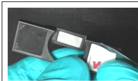
Peel the backing from the adhesive magnet protection
