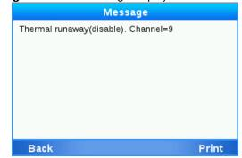
With **cobas**<sup>®</sup> **Liat**<sup>®</sup> Software v3.3.0, this error occurs at the first instance of thermal runaway. If the instrument is not powered off using the 'shut down' option located on the log on screen followed by pressing the power button, subsequent runs will not show the error message and may not abort, and a high rate of assay invalids and/or some false positives may occur.
