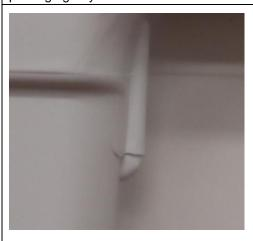
Not conform: Crack in intellipack packaging tray
