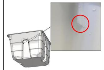
Area on the intellipack packaging tray where the failure was detected with crack
