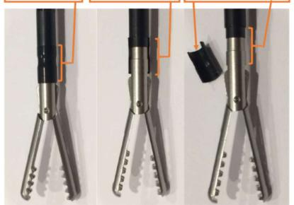
The heat-shrink tube remains in one piece but gives the appearance that a longitudinal portion is missing. This is because after splitting it shrinks in size to expose a portion of the metal tip (see picture below). If a split occurs, the heat-shrink could detach from the device before or during surgery and, if cautery is needed, there is the potential for burn due to insulation failure.
