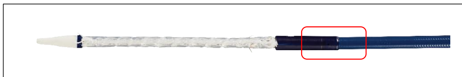
Figure 1. Example TBE SB device on catheter, red box showing location of catheter separation.
